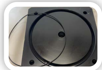
Figure 8 End Seal installation in Reservoir Cap
