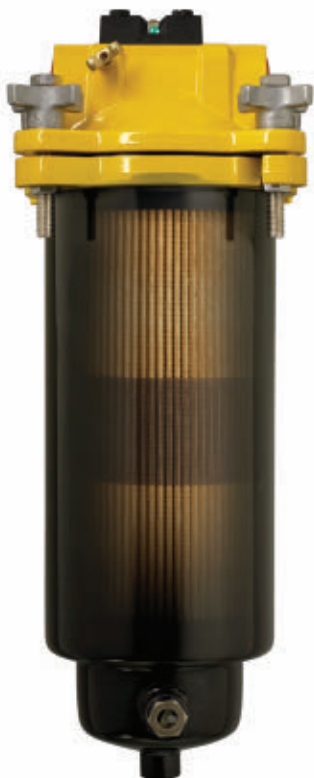
Parker Racor's FBO fuel filter and water separator assembly is designed for fuel dispensing pumps or as a primary fuel filter and water separator on a large diesel engine, or in bulk fuel handling, fuel transfer and other higher flow applications.
