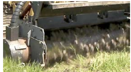
Figure 1: RotoSlasher units feature Parker's P24 GOLD CUP pump teamed to a CAT 18 525 hp industrial diesel engine, powering two 180cc bent axis motors
