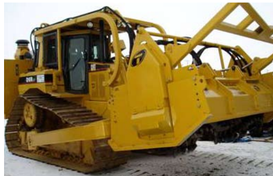
Figure 1: RotoSlasher units feature Parker's P24 GOLD CUP pump teamed to a CAT 18 525 hp industrial diesel engine, powering two 180cc bent axis motors
