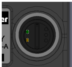
Figure 25: The Micro SD card slot in the rear side of the Pro Display unit. In normal operation and final installation, the slot shall be always protected with a cover plug. Cover plug is part of Pro Display unit assembly.
