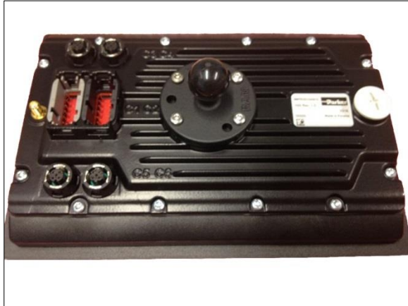
Figure 21: Figure A - RAM ball installed into rear side of Pro Display. Figure B - Swivel mounting accessory attached into Pro Display before final install into vehicle.
