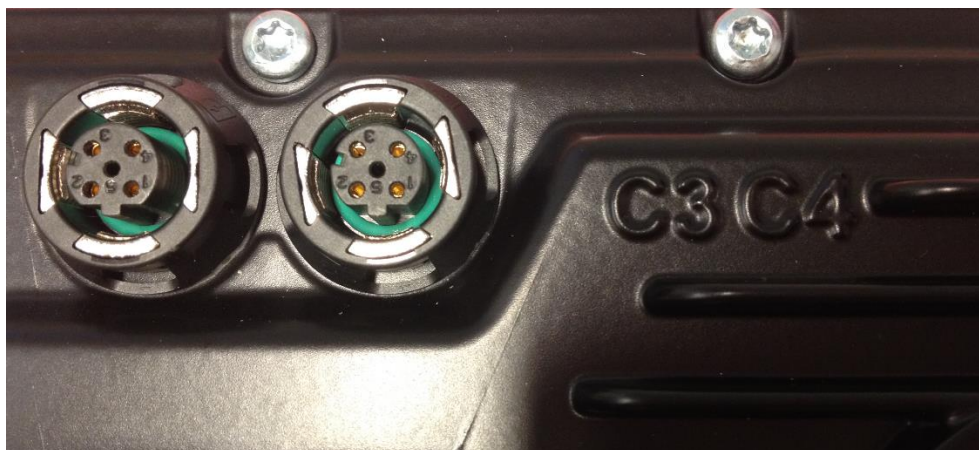
Figure 24: USB Connectors C3 & C4 on the backside of the module
