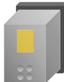
Drive mounted on a “footprint” filter
