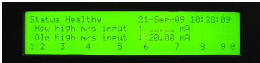
Figure 4.1.4.3.7 Input the New high m/s input Screen
