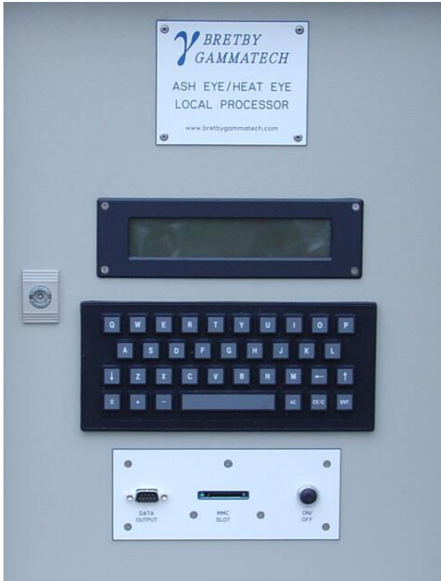
Figure 1.1 Local Processor Inner Door
