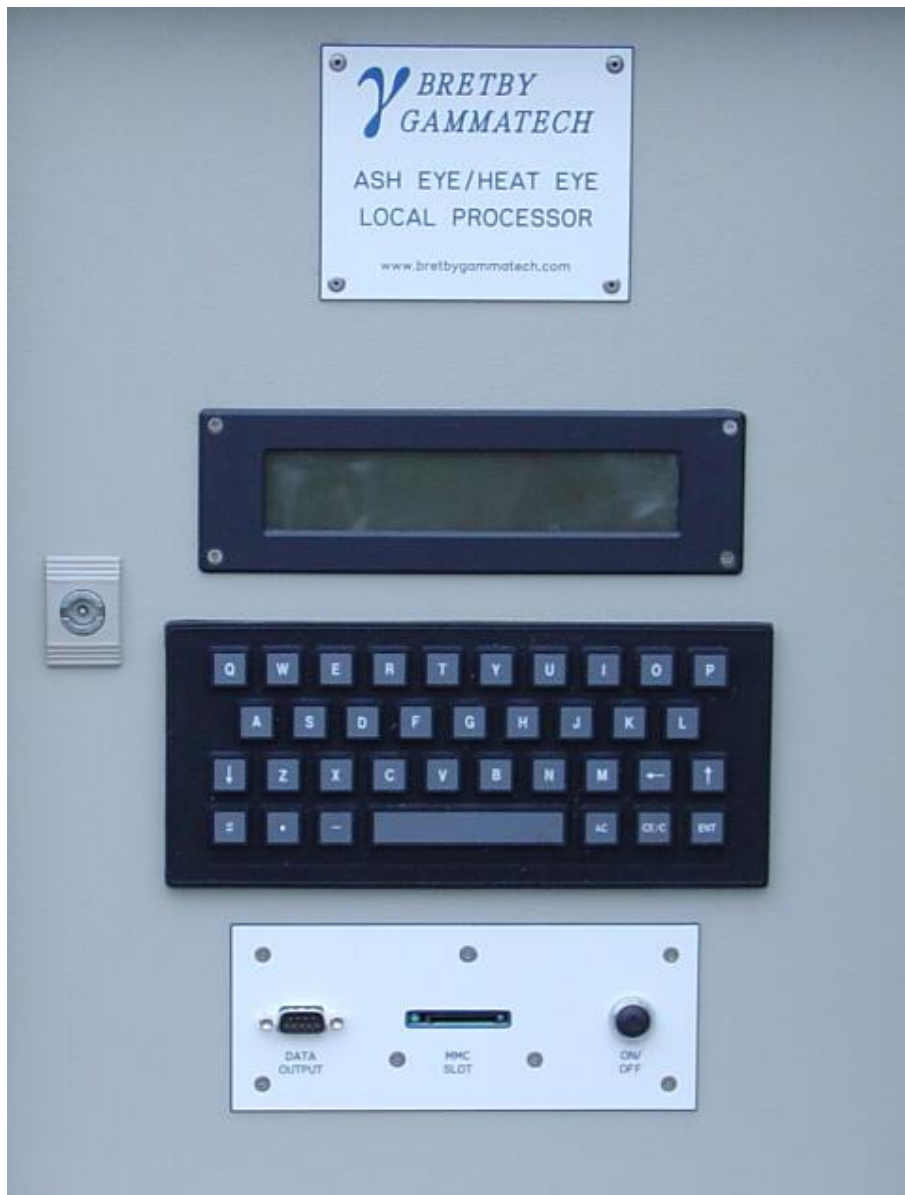
Figure 1.1 Local Processor Inner Door
