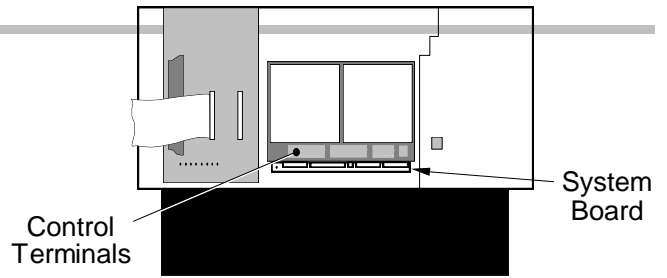
BOTTOM WITH TERMINAL COVER REMOVED
