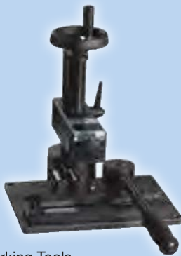
TH3E-EM6-M Hose Cutting Machine
