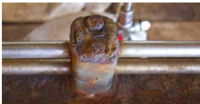
Crevice corrosion between the tube/tube trap interface.
