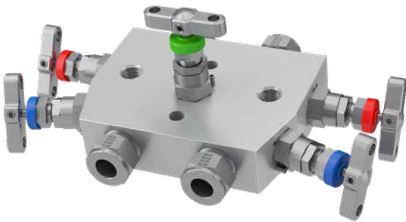
Example shown: 5-valve remote/line mount manifold featuring the Parker A-LOK® Superior Advantage Inverted integral tube fitting connections for the impulse line and NPT ported connections for the vent/drain.
