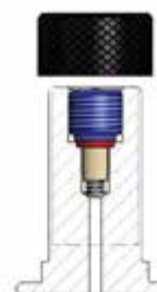
Model of valve stem integrated 5/8" 18 UNF (D)
