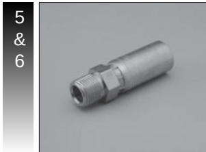
Verify fitting part number(s) match work order. Visually inspect fitting(s) for a through-hole, threads and damage.
