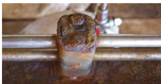
Crevice corrosion between the tube/tube trap interface.
