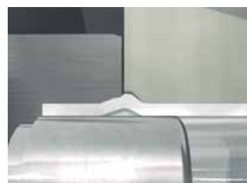
The inner contour also gets slightly deformed but remains smooth and unrestricted for good flow characteristics
