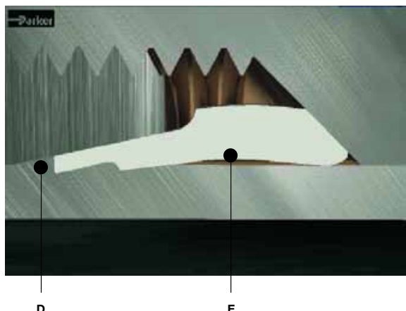
After tightening the nut
