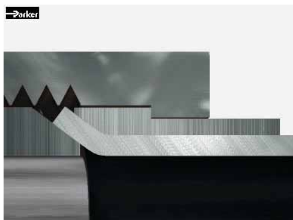
After tightening the nut
