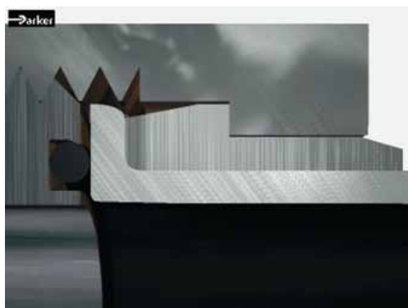
Before tightening the nut
