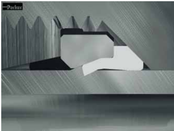
After tightening the nut
