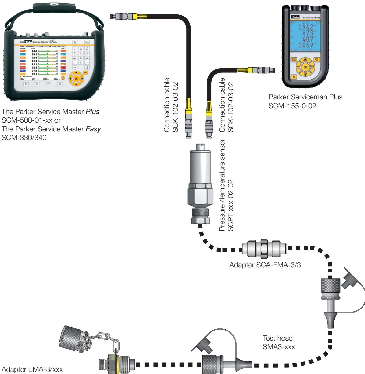
**Pressure/temperature measurement SCPT**
